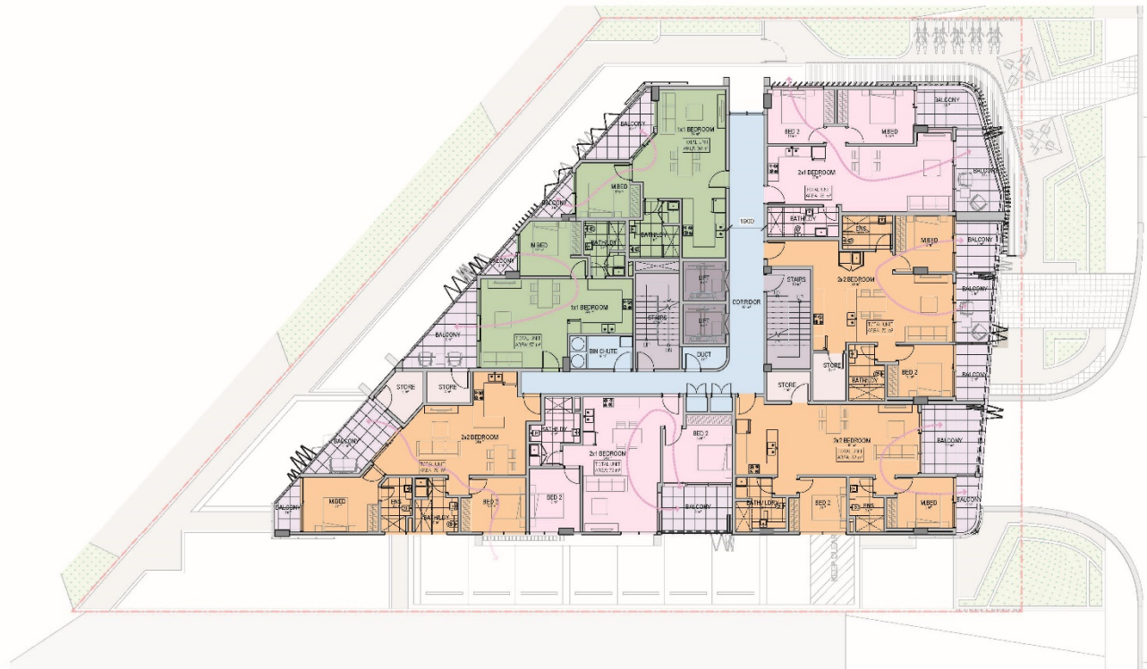
1 TYPICAL FLOOR PLAN LEVEL 3 - 10 1:100 TOTAL FLOOR AREA: 730 #2 FLOOT PLATF AREA (INCLUDING UNENCLOSABLE BALCONIES): 608 #2 UNENCLOSABLE BALCONIES: 102 #2
